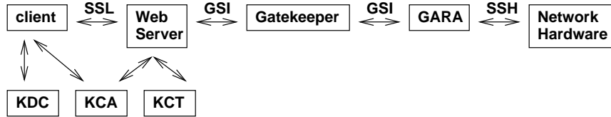
Fig. 1. KX509 GARA Web Interface. This figure shows how local network resources are reserved with the GARA Web interface. KX509 junk keys replace long term PK credentials. Communications with the KDC, KCA, and KCT are Kerberos protected.
