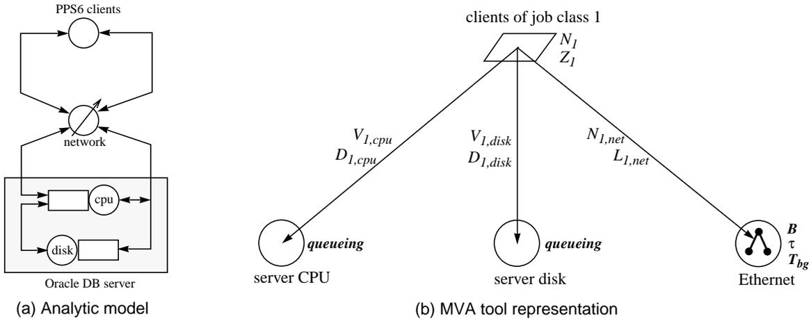
Figure 2. Queuing network model of the two-tiered PPS6.
