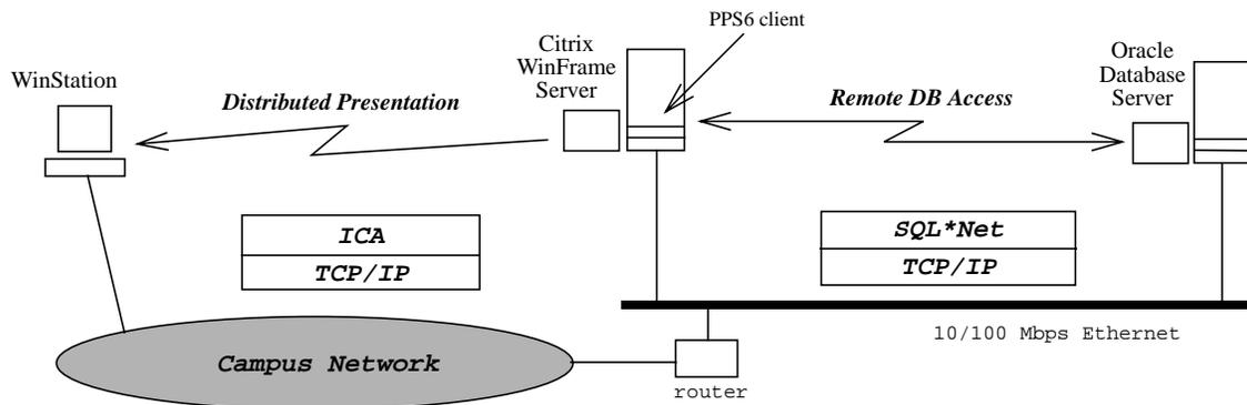
**Figure 1.** The production deployment of PPS6 with Citrix WinFrame extension.
